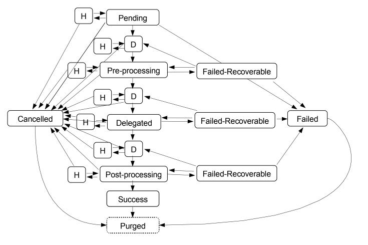
D – delayed. Although all tasks in previous state are finished Activity can't proceed to next state due to some internal reasons. For example saturation of available resources. This can be either separate states (per every delayed state) or sub-state.
