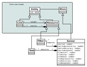
The **Filter** subtypes the **Resource**, with no attributes It is a component of the **Sensor** It provides a hook for provider specific aggregated metrics (aka SLO)
