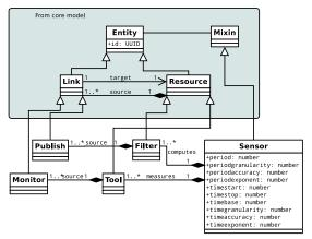
The **Publish** subtypes an OCCI **Link**The sources of the link are **Filters**, the target is a SLA-specific **Resource** (not shown in the figure)
