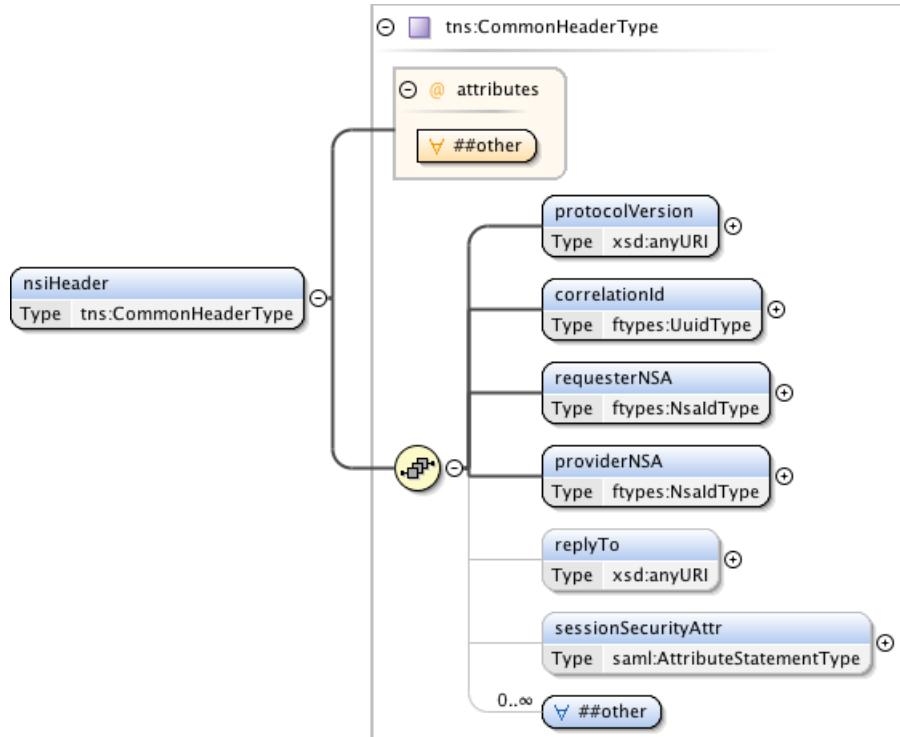
**Figure 1 – Common NSI 2.0 framework message header.**
